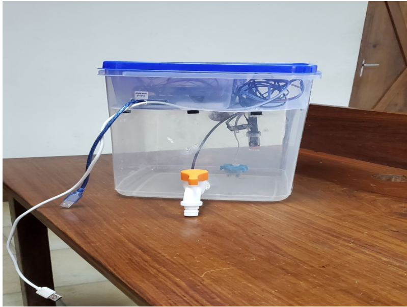
Figure 5: Assembled sensing subsystem prototype comprising Arduino Mega, NodeMCU, and connected sensors
