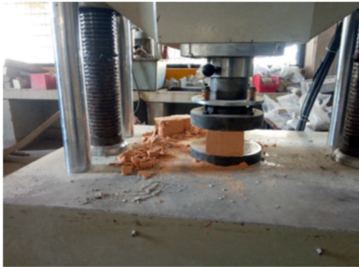
A Brick sample on a universal test
