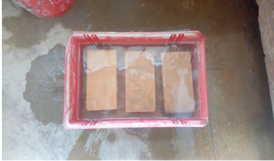
Plate 2: Submerged bricks in water to determine water absorption
