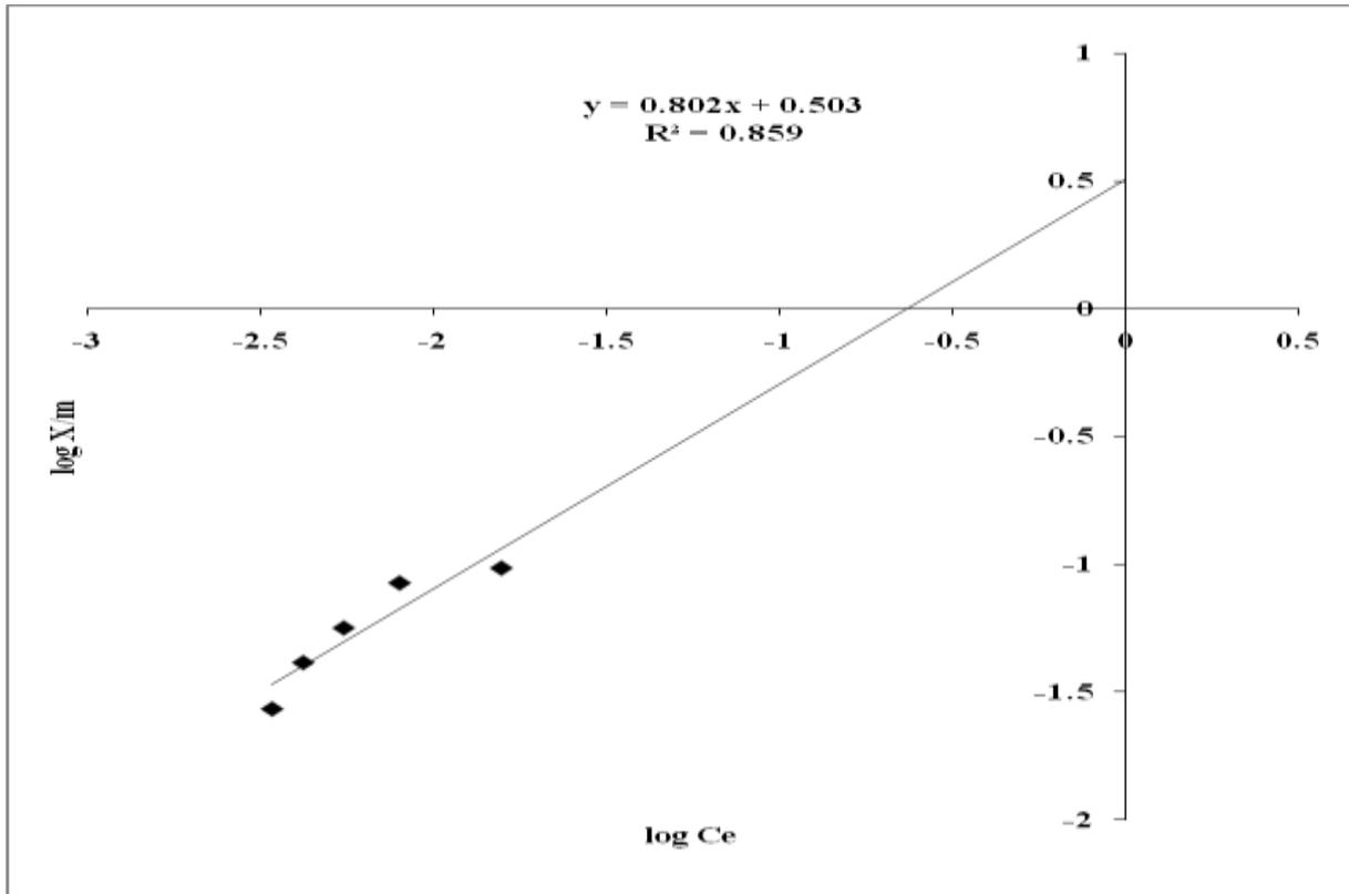
Figure 8 Freundlich adsorption isotherm for removal of Lead at pH= 7
