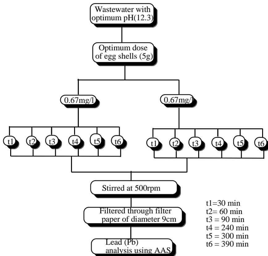
**Figure 2** Batch Experiment layout, Effects of Contact time
