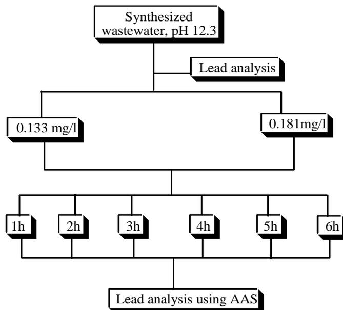
**Figure 3** Column experiment layout, Effect of contact time and initial concentration
