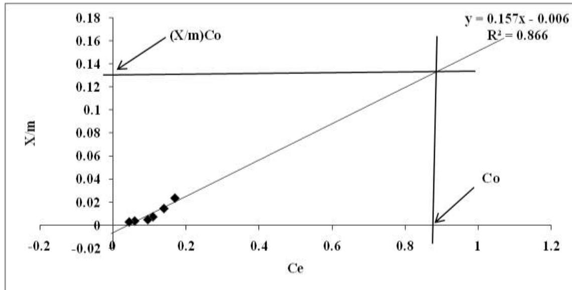
Figure 12 Adsorption capacity of Lead removal at pH 12.3
