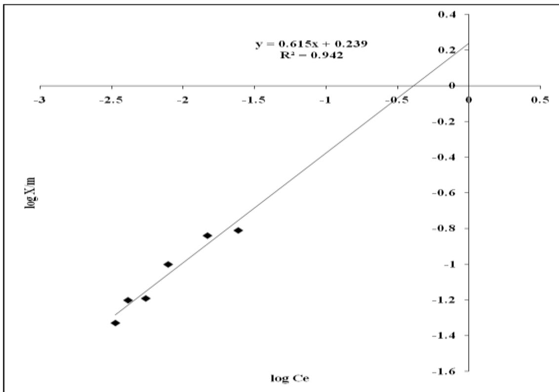
**Figure 7** Freundlich adsorption isotherm for removal of Lead at pH= 3.3
