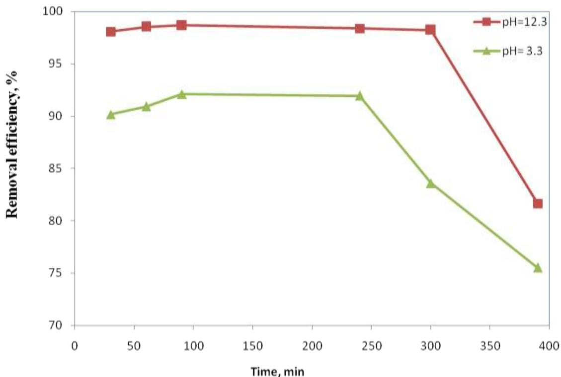
**Figure 6** Effect of contact time on lead removal
