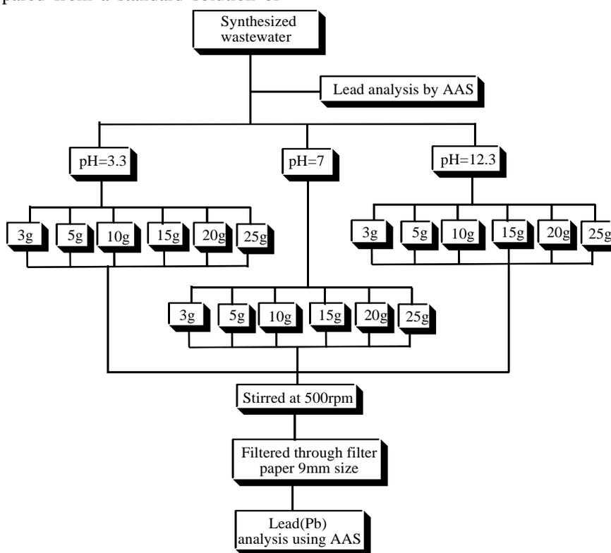
Figure 1 Batch experiment layout, effect of dose and pH on the removal of lead.
