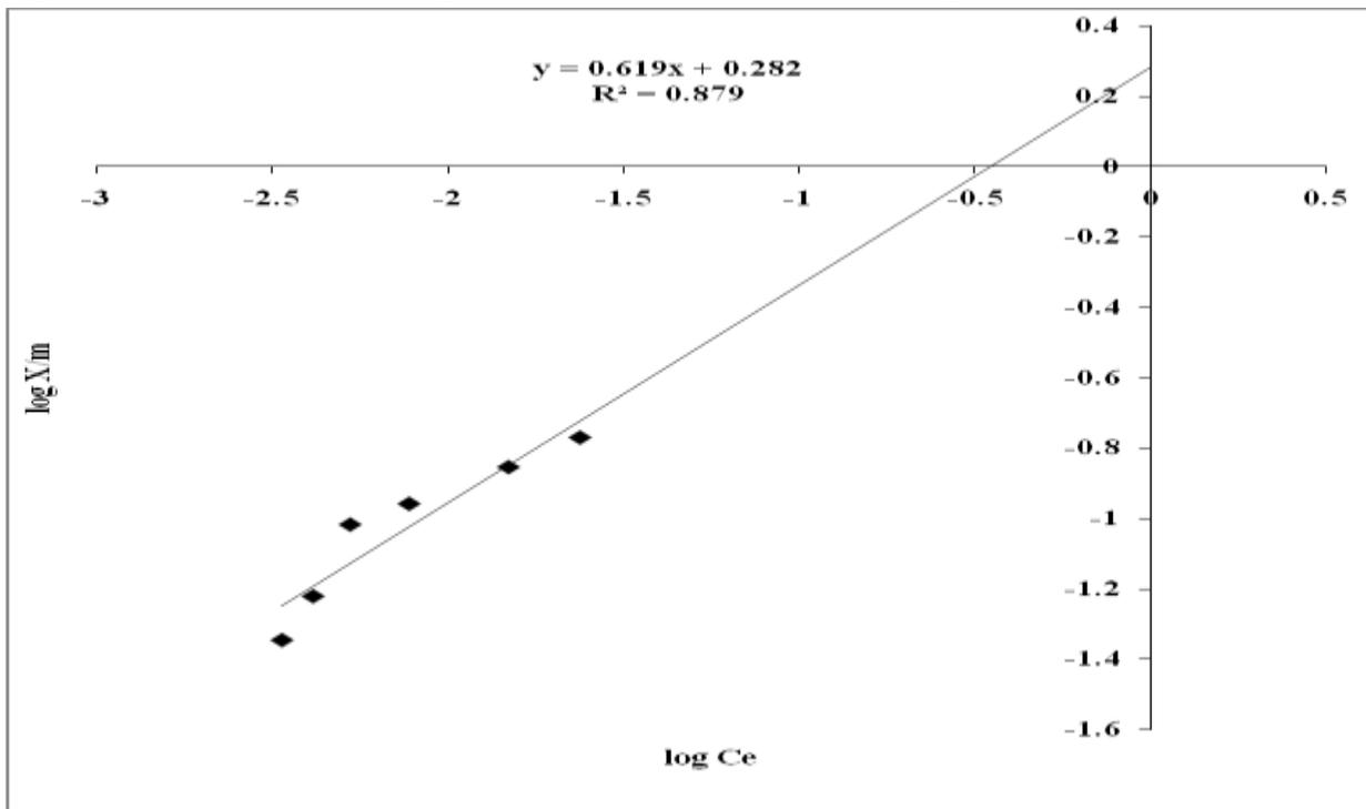
Figure 9 Freundlich adsorption isotherm for removal of Lead at pH=12.3
