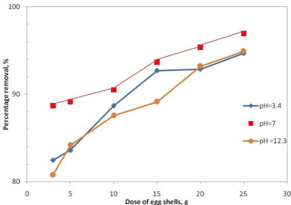
**Figure 5** Effect of Dose of egg shell at different pH
