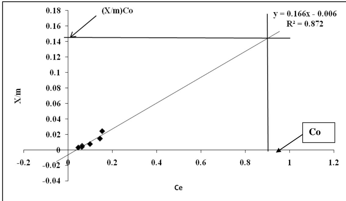
**Figure 10 Adsorption capacity of Lead removal at pH 3.4**
