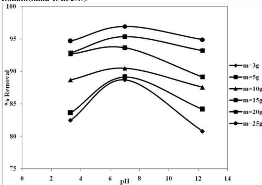
Figure 4 Effect of pH on Lead removal with different egg shell doses
