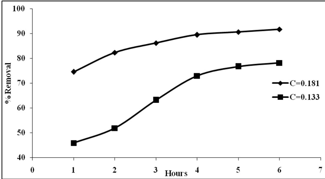
**Figure 13 Effect of initial concentration on time for removal of Lead**
