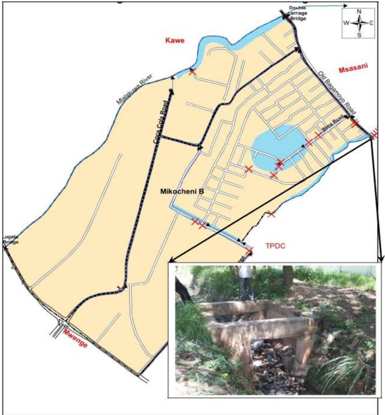
**Appendix 3: Proposed drainage channels to facilitate the drainage network**
