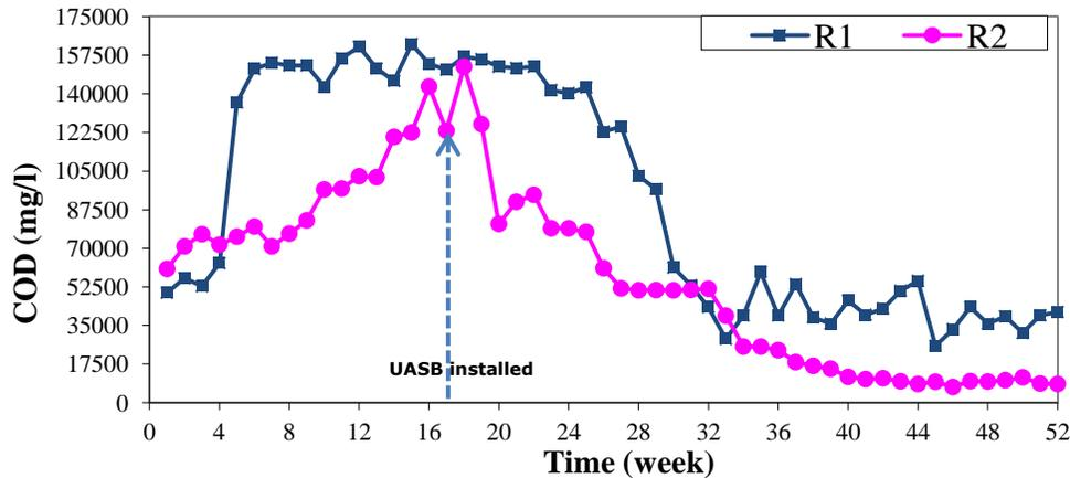
**Figure 3:** COD concentrations in leachate of R1 (control) and R2 (simulated LFB) as a function of time
