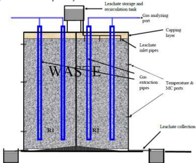
Figure 1: Schematic representation of the pilot scale LFB
