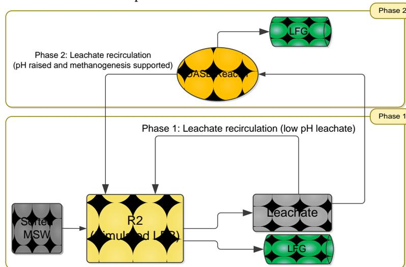
**Figure 2: Flow diagram phase 1 and 2 of R2 (simulated LFB)**
