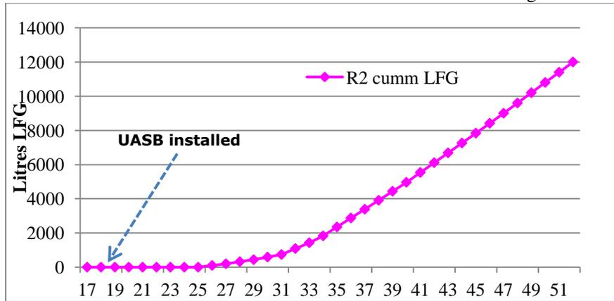
**Figure 8:** Cumulative LFG volume from UASB reactor coupled to R2 (simulated LFB)
